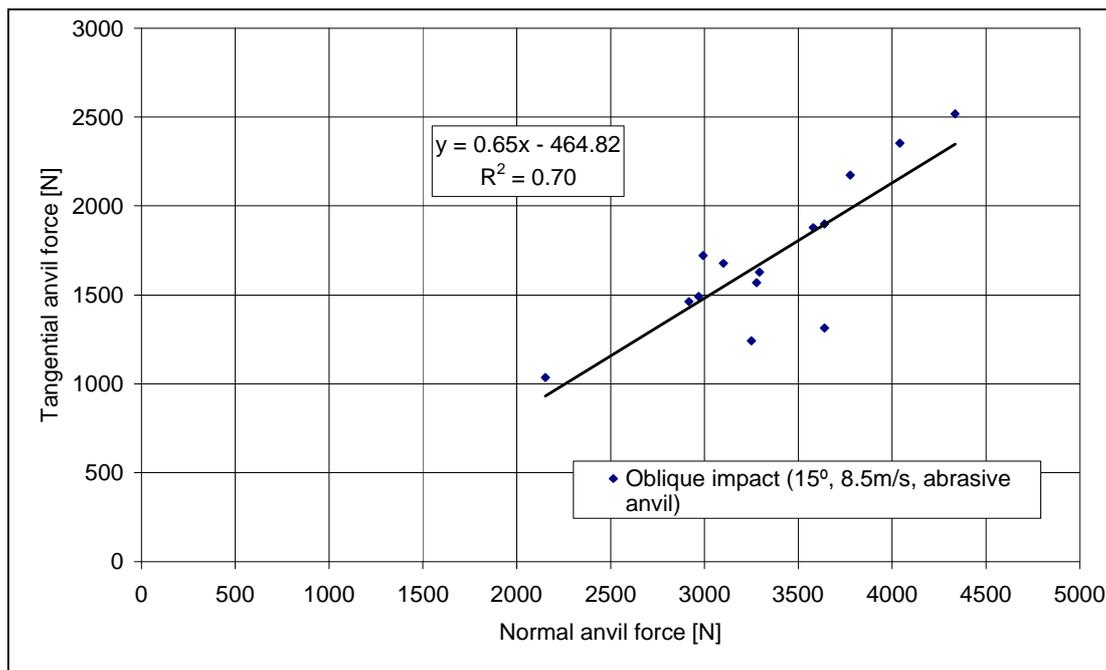
**Figure 9 Relationship between tangential and normal anvil force for 8.5m/s oblique impacts**
