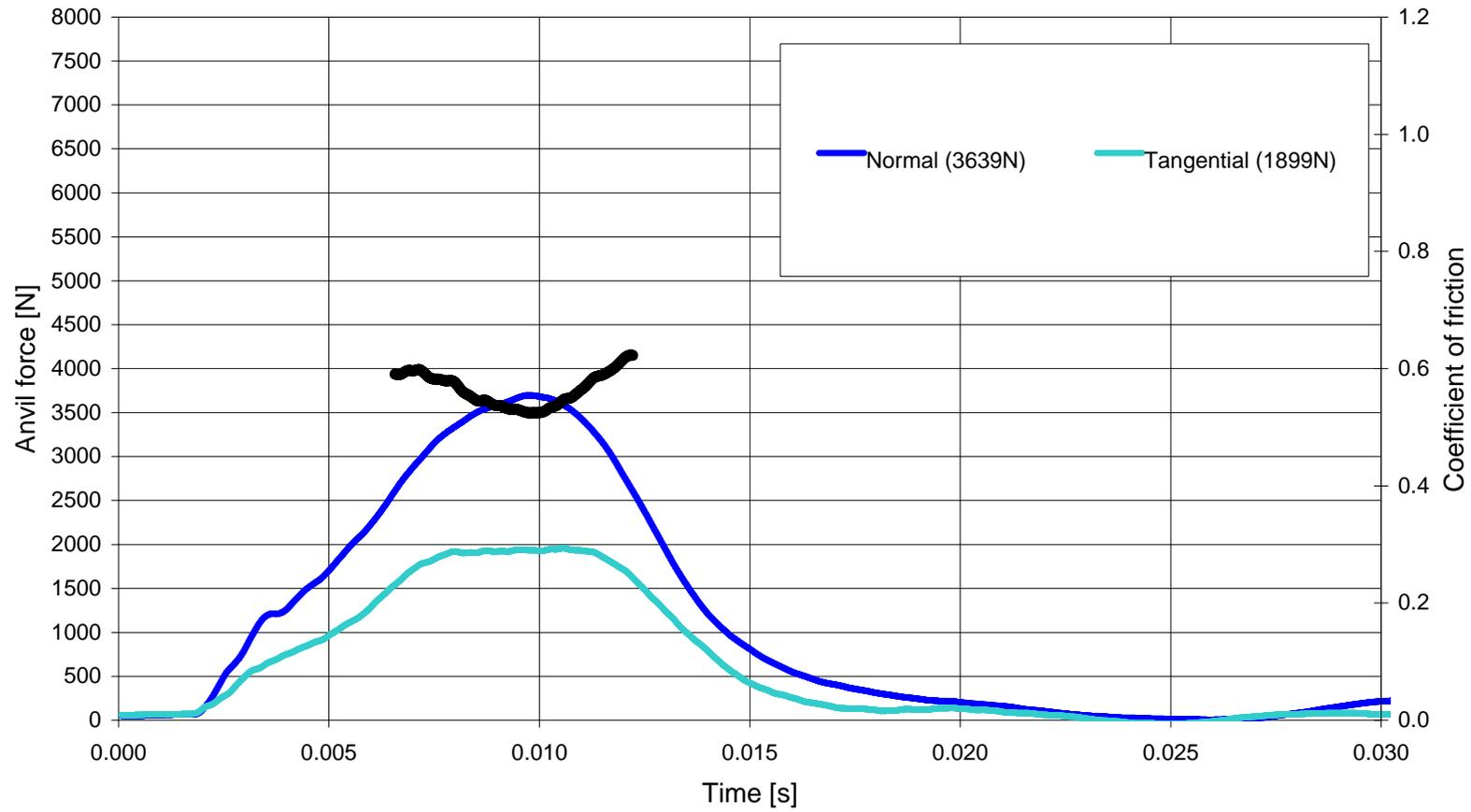
3a helmet [Side R] equipped with a Reg22 headform onto 15° Oblique at 8.5m/s (e08lz)
