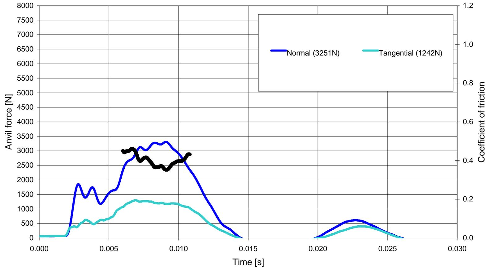
3a helmet [Side L] equipped with a Reg22 headform onto 15° Oblique at 8.5m/s (d08lz)
