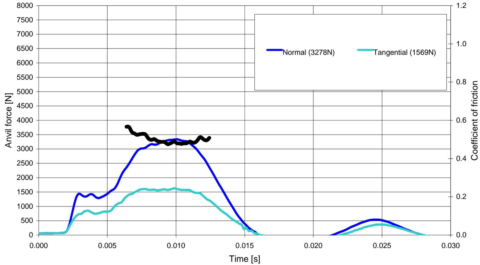
5a helmet [Side R] equipped with a Reg22 headform onto 15° Oblique at 8.5m/s (e11lz)
