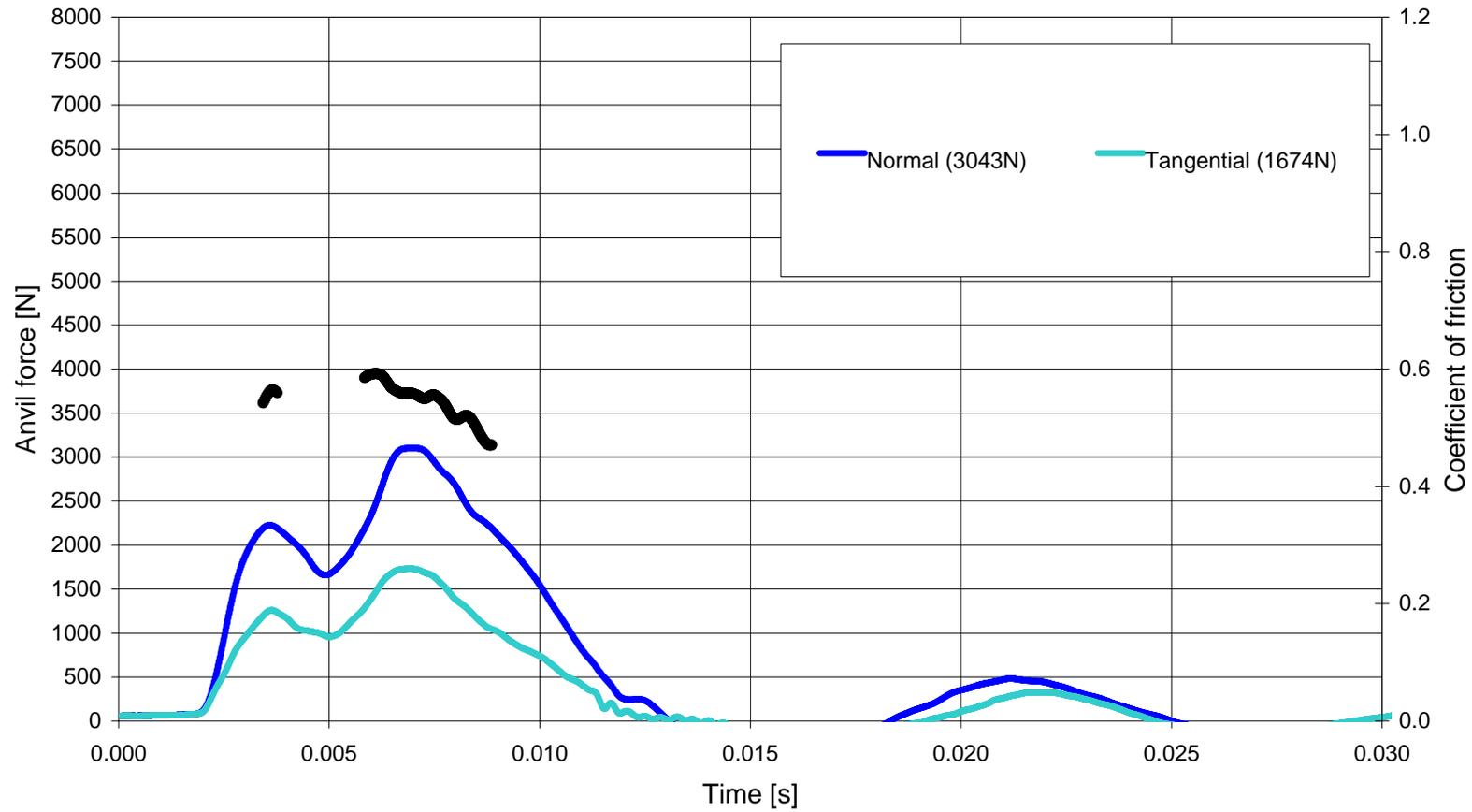
2a helmet [Side L] equipped with a Reg22 headform onto 15° Oblique at 8.5m/s (b111z)
