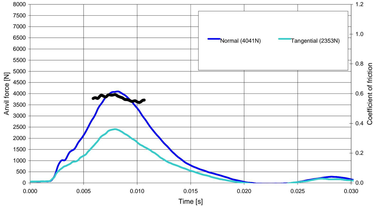
4a helmet [Side R] equipped with a Reg22 headform onto 15° Oblique at 8.5m/s (h08lz)
