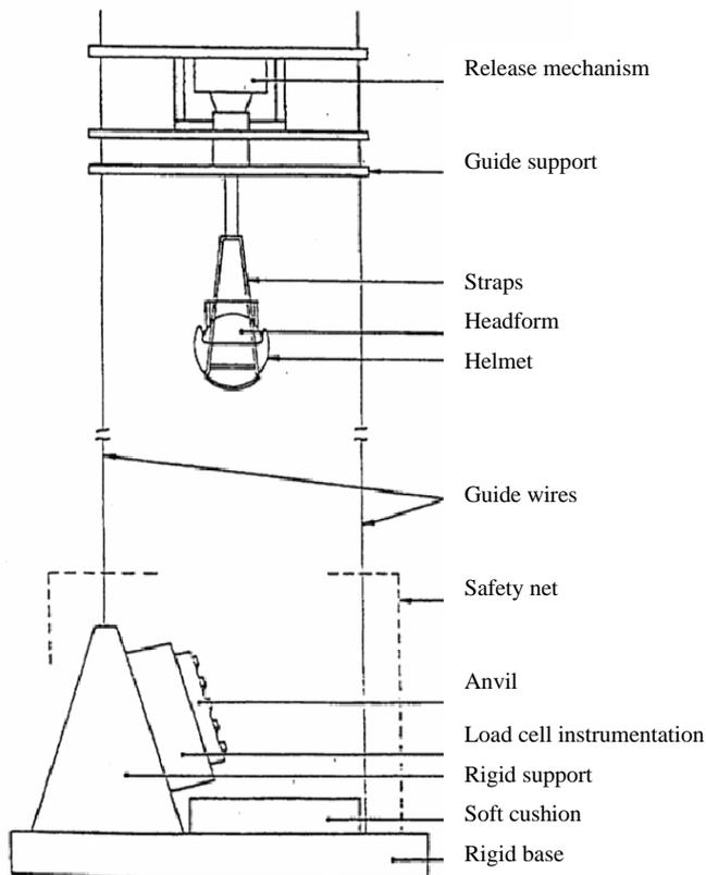
**Figure 2. UN ECE Regulation 22.05 method A test apparatus**
