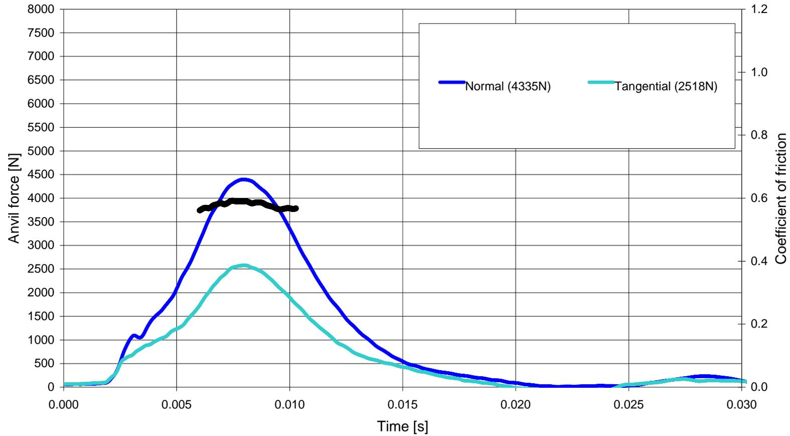
5a helmet [Side L] equipped with a Reg22 headform onto 15° Oblique at 8.5m/s (i08lz)
