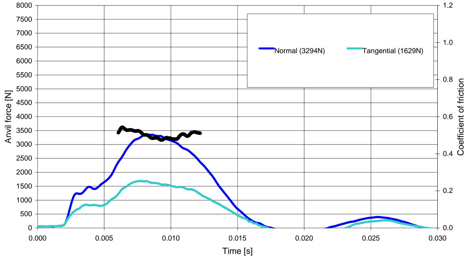
2b helmet [Side L] equipped with a Reg22 headform onto 15° Oblique at 8.5m/s (k08Iz)
