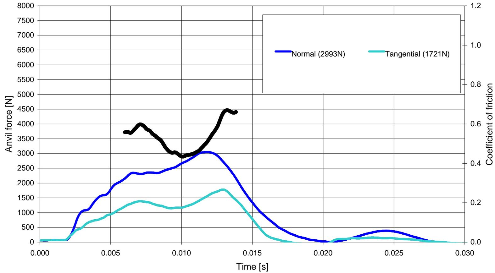
2a helmet [Side L] equipped with a Reg22 headform onto 15° Oblique at 8.5m/s (a08lz)
