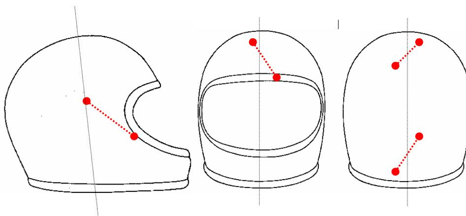
**Figure 4 Orientation of the kerb anvil for linear impact tests**
