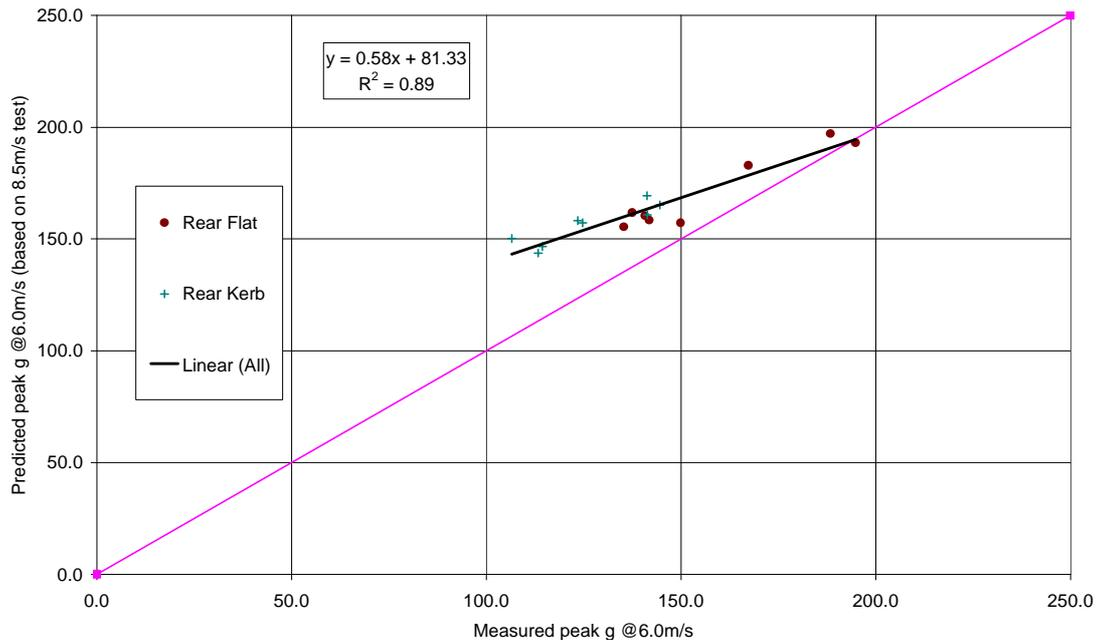
**Figure 14. Comparison of predicted and measured acceleration for 6m/s impacts for rear impact site**
