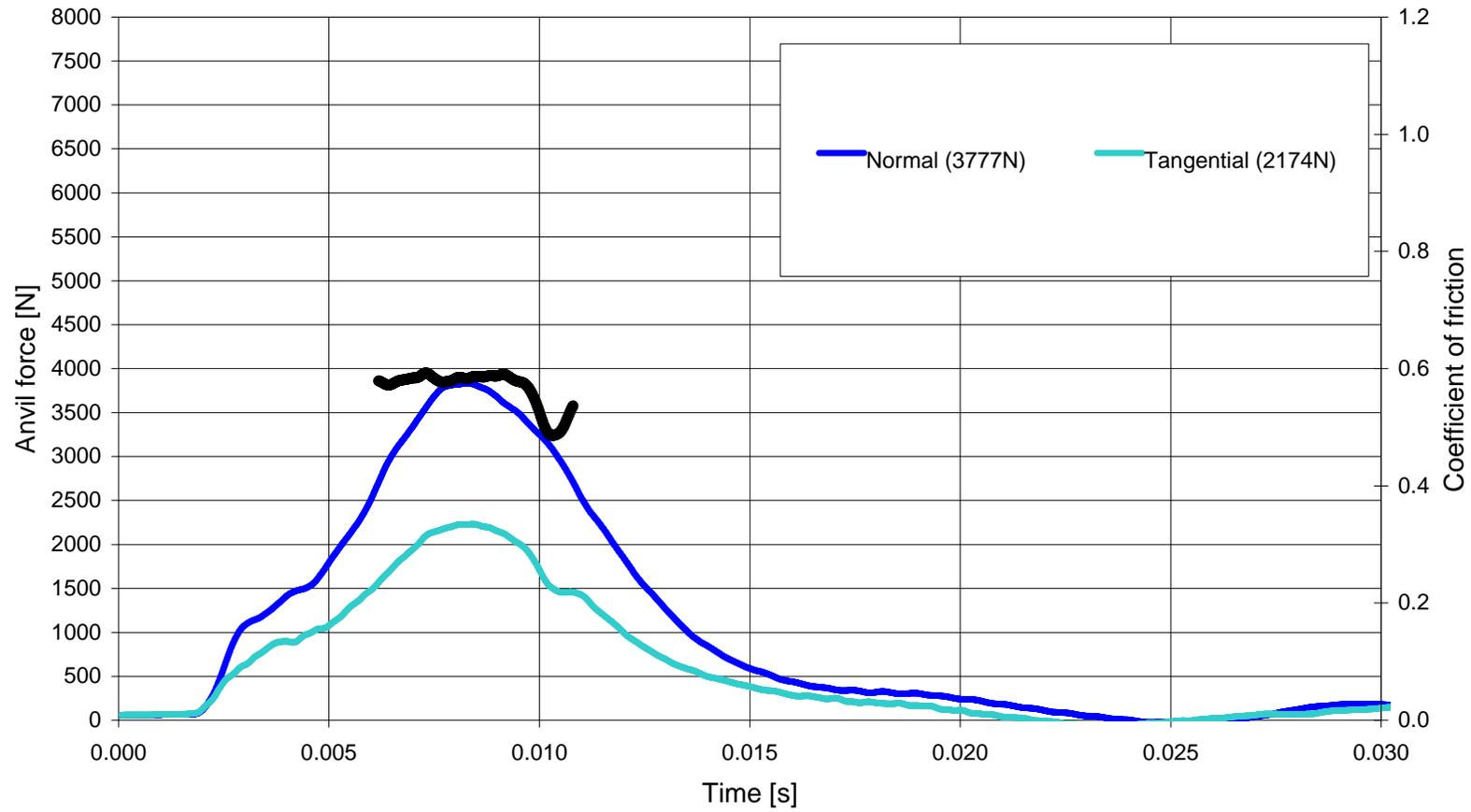
4a helmet [Side L] equipped with a Reg22 headform onto 15° Oblique at 8.5m/s (f08lz)
