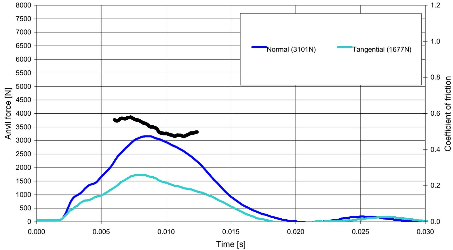
1a helmet [Side L] equipped with a Reg22 headform onto 15° Oblique at 8.5m/s (h01lz)
