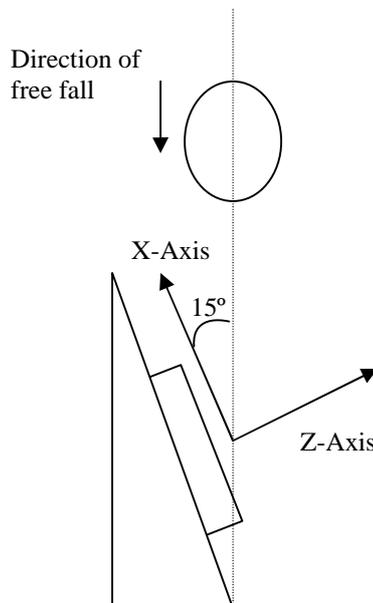
**Figure 3(b) Configuration of oblique anvil test**
