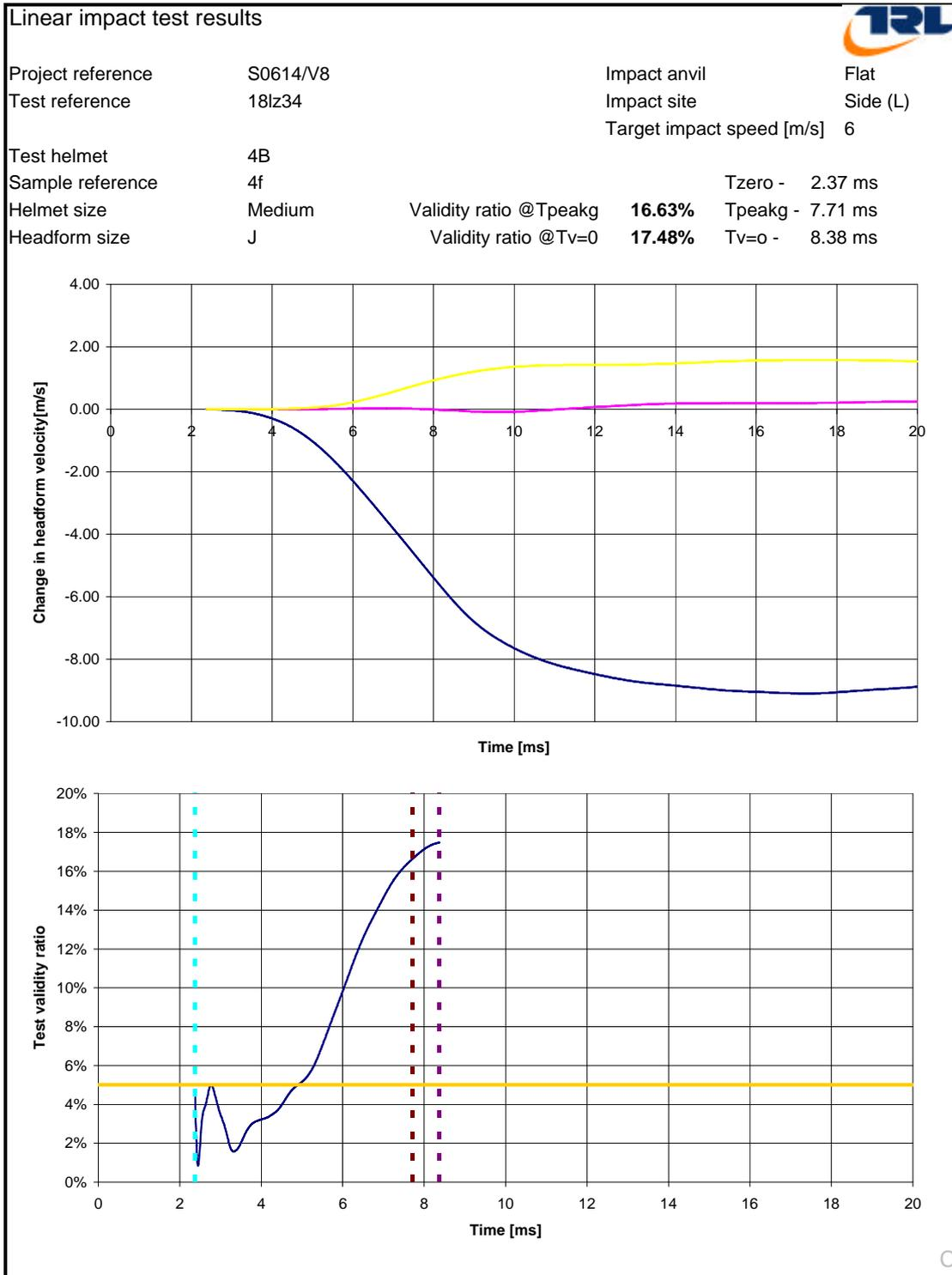
**Figure 7(b) Typical test results and validity ratio visualisation**
