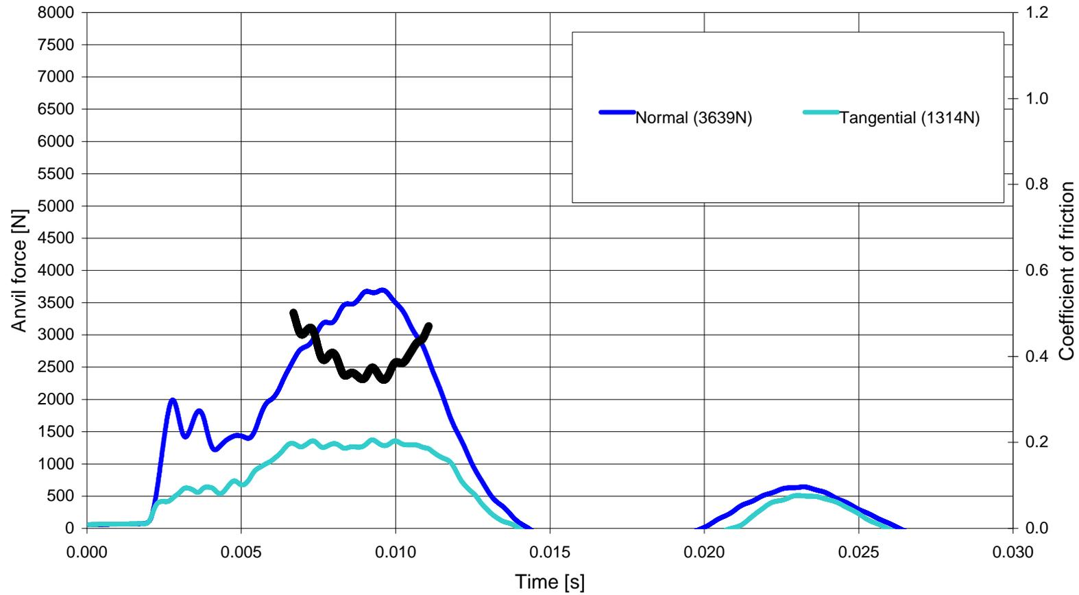
2a helmet [Side R] equipped with a Reg22 headform onto 15° Oblique at 8.5m/s (b08lz)
