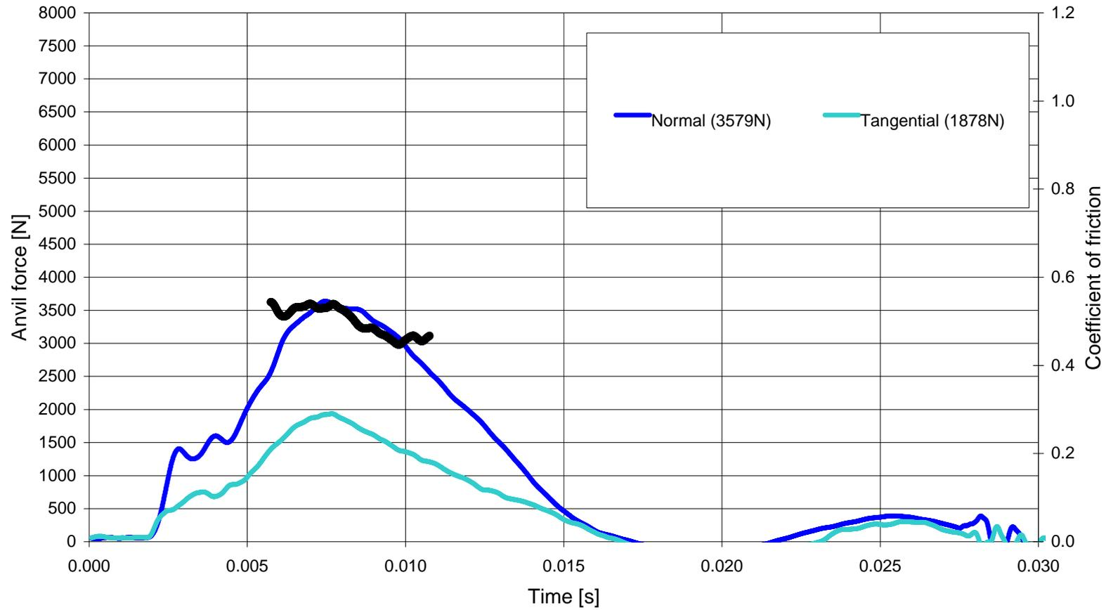
5a helmet [Side R] equipped with a Reg22 headform onto 15° Oblique at 8.5m/s (j08lz)
