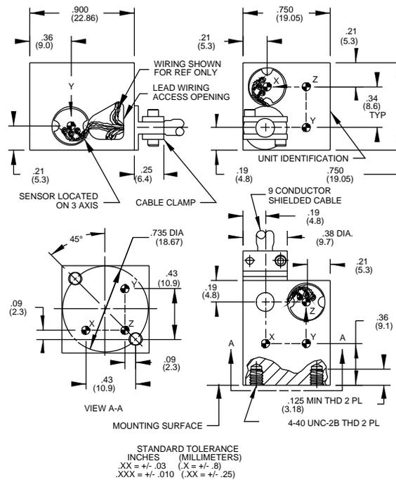
ENDEVCO Model 136 Three-Channel System, Model 4430A or OASIS 2000 Computer-Controlled System are recommended as signal conditioner and power supply.
