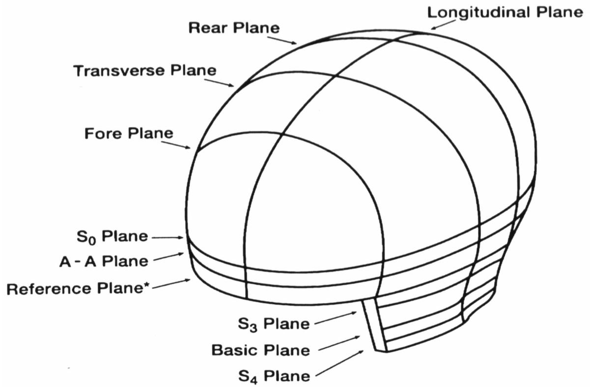
Figure A1. ISO DIS 6220 test headform
