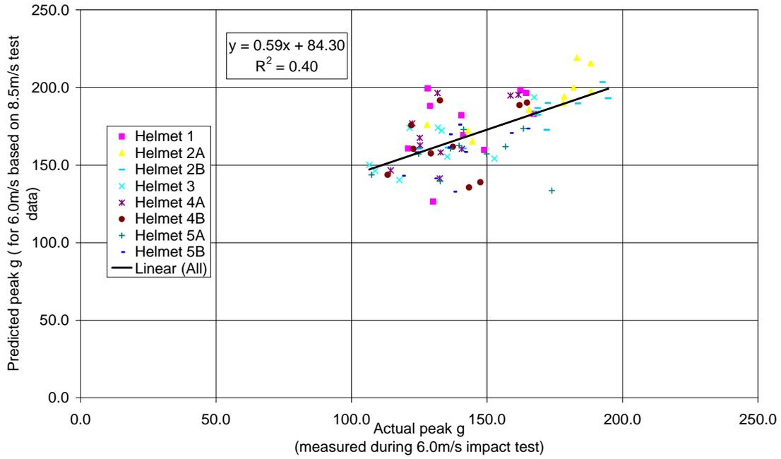
**Figure 13 Comparison of predicted and measured peak acceleration for 6.0m/s helmet impacts**
