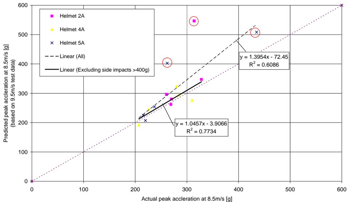
**Figure 12 Comparison of predicted and measured peak acceleration for 8.5m/s helmet impacts**
