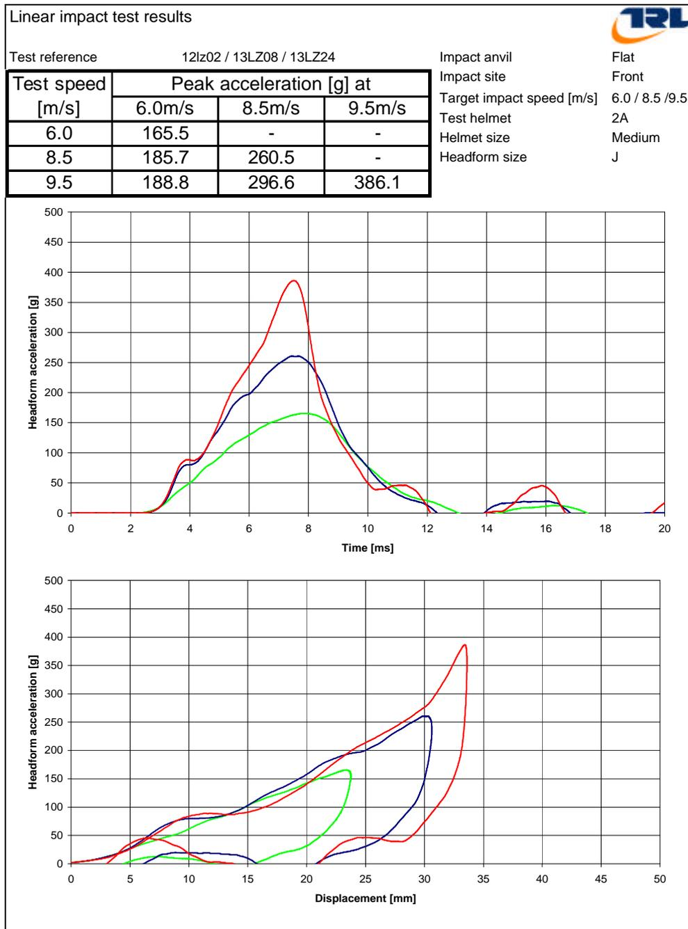
**Figure 11 Illustration of acceleration – displacement curve for three helmet impact tests onto a flat anvil and differing speeds**
