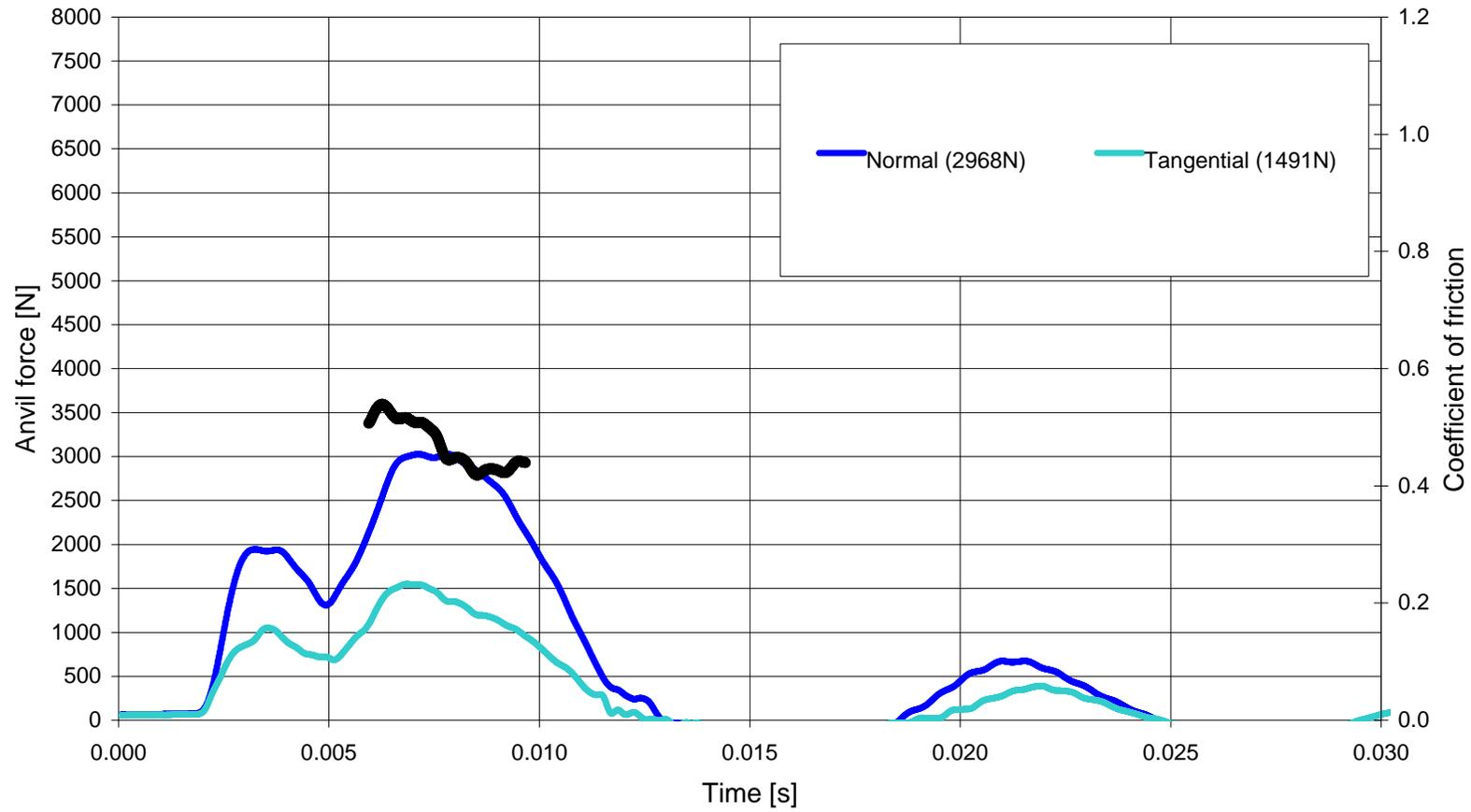
5a helmet [Side L] equipped with a Reg22 headform onto 15° Oblique at 8.5m/s (d111z)
