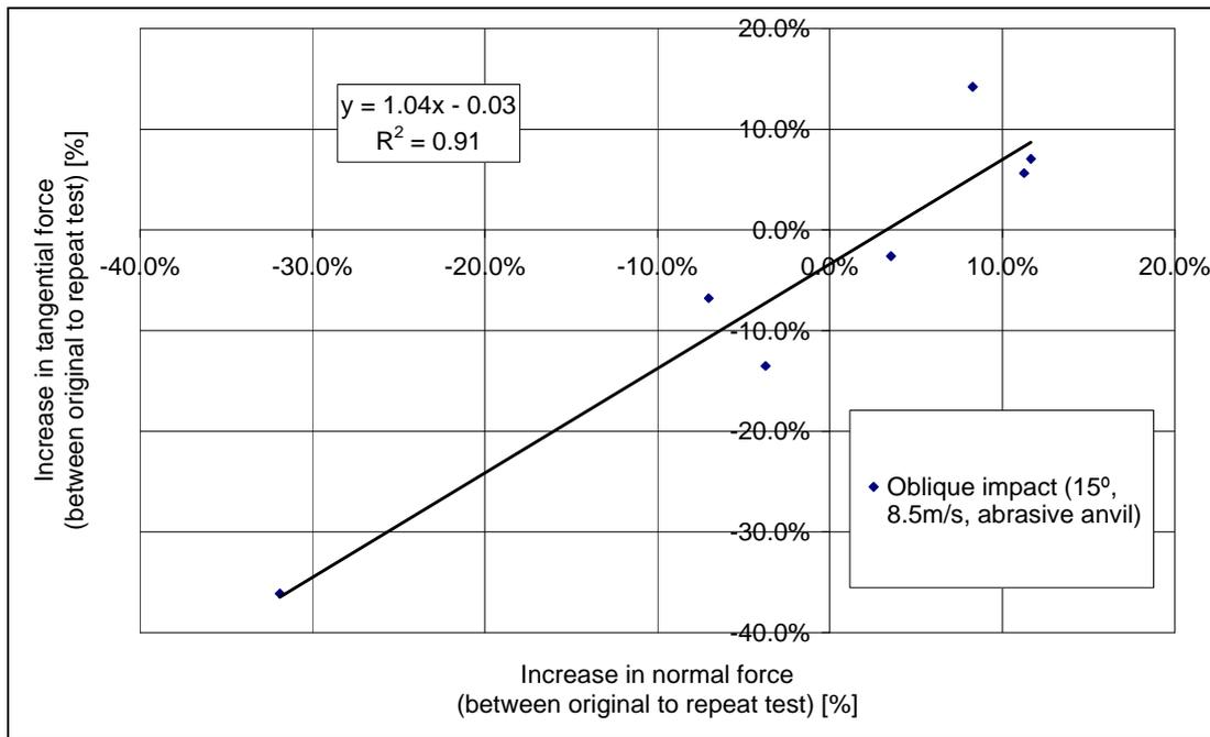
**Figure 10 Relationship between change in tangential and normal anvil force for comparable (original and repeat) 8.5m/s oblique impacts**
