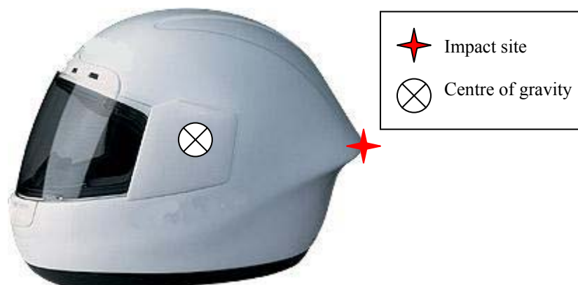
Figure 5.14. Helmet with sculptured shell design (approximate centre of gravity and rear impact site positions shown)
