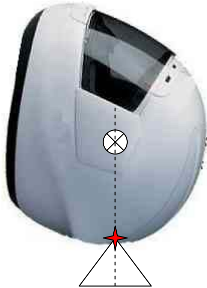
Figure 5.13. Conventional helmet in impact configuration (centre of gravity aligned with impact site)
