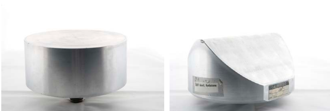
Figure 2. Flat and Kerb Impact Anvils
