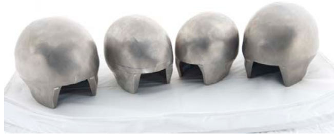
Figure 3. Three quarter head forms for linear impact testing.
