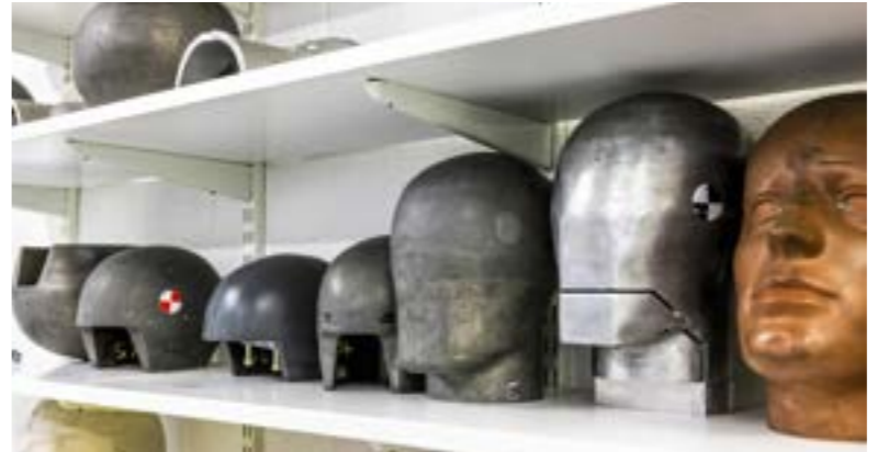
Sensor-laden headforms replicate the human skull during impact testing
