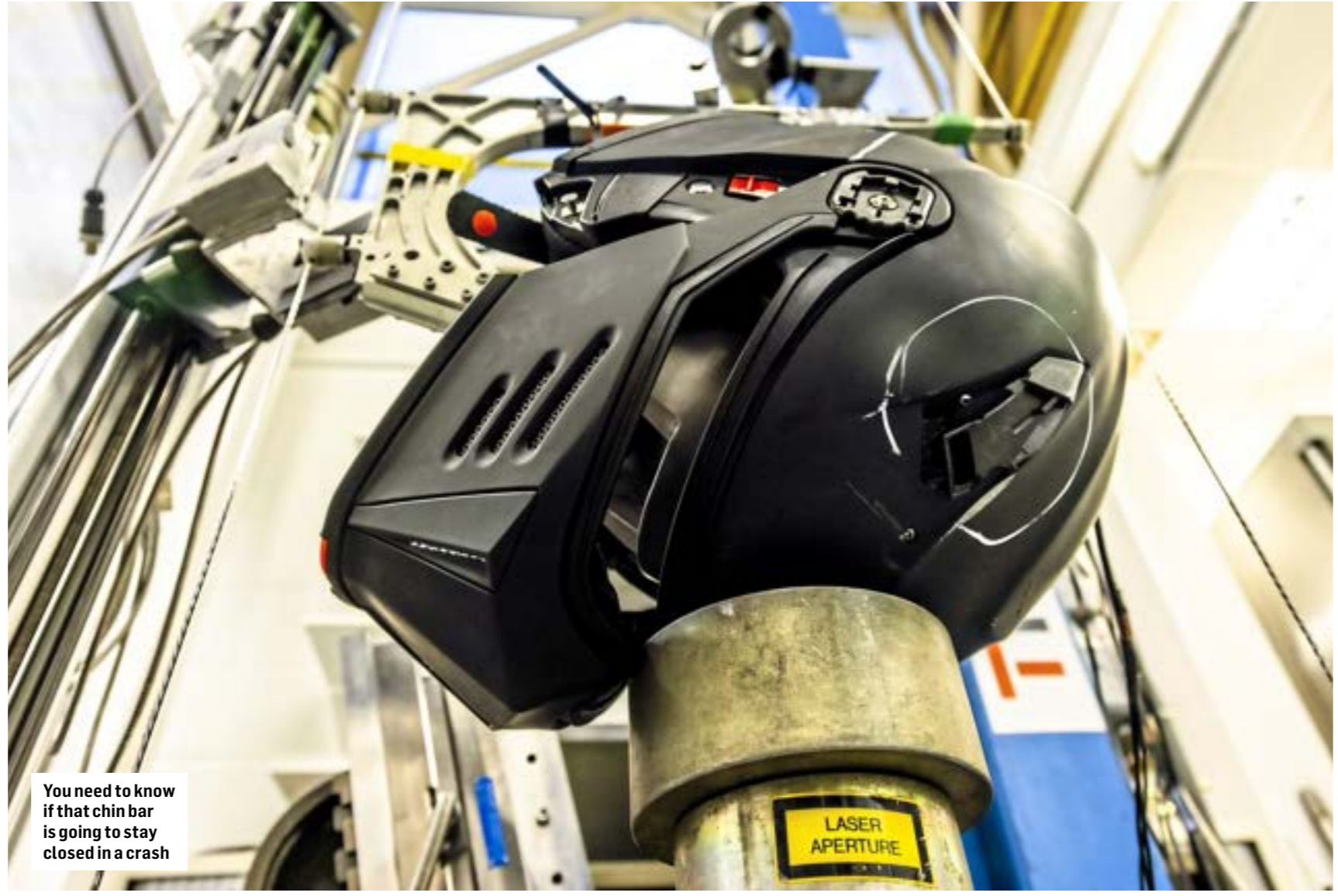
Sensor-laden headforms replicate the human skull during impact testing
